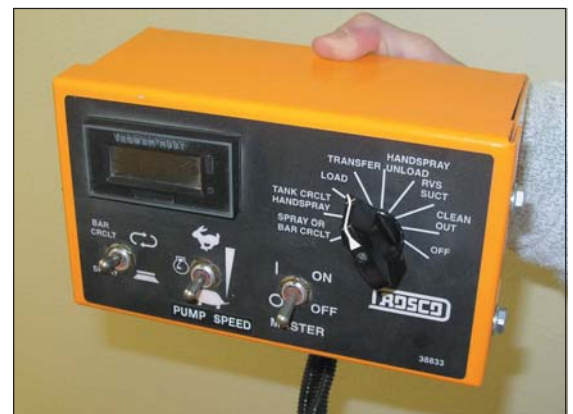
In-cab controller box controls gallons-per-minute, rotary valves, and spraybar on/off/bar circulate from the towing vehicle.
