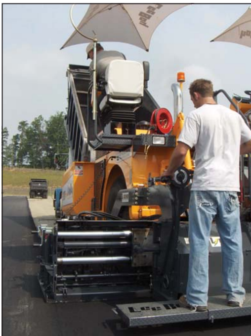
Slide-Out operator station and extendible walkboard provides the paver operators with enhanced visibility.
