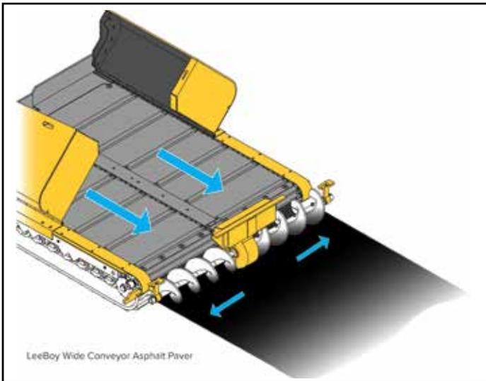
As the mix moves from the front of the hopper to the rear of the paver, machine vibration and the shearing forces of the conveyor slats begin to break down the composition of the mix. The faster the conveyors run, the greater the risk of separation. The same is true of the auger speed. The goal is to minimize the shearing forces on the mix while maintaining a consistent head of material in front of the screed.
