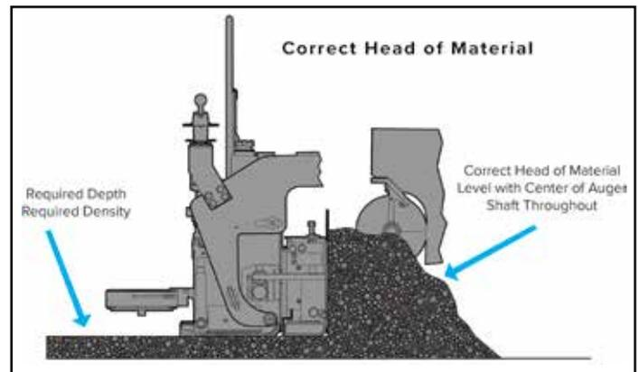
The consistency of the material head, including its total volume and depth is determined in large part by the paver speed and material flow rate. Of these, maintaining a constant paving speed is especially critical.
